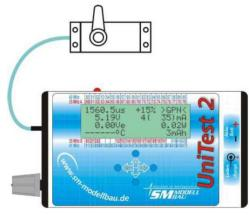
The diagram to the left shows the proper connection of a servo when performing servo test. а The servo can be connected to "Servo 1" or "Servo 2". You can also connect two servos at the same time. In this case the current consumption displayed by UniTest 2 is the total current consumption of both servos combined. When connected like this, the servos are powered using UniTest 2's internal battery. This battery has four cells and is comparable to а standard receiver battery.
