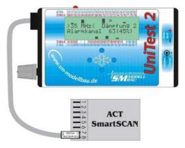
The diagram to the left shows how to connect a SmartSCAN scan receiver.
