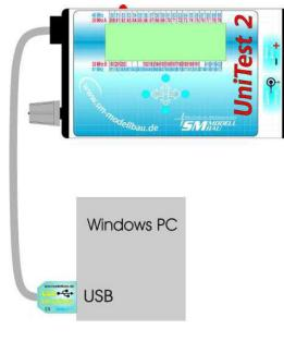
Connect the **USB-Interface** to a free USB port on your PC. Connect the other end to the "*Seriell 1 COM*" connector of the **UniTest 2.**
